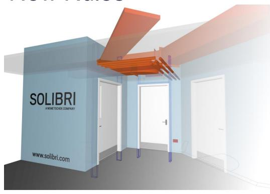
Stud Opening Rule Checks for clearances for services above doors against items that are not typically modelled Door Leading Edge Rule
