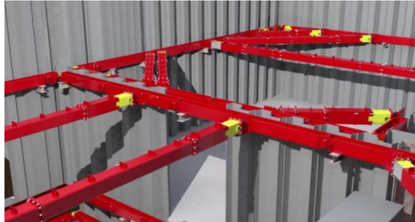
Cofferdam BIM model and frame
