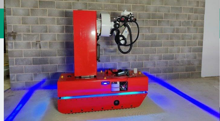
Skanska's Collaborative On-Site Construction Robot
