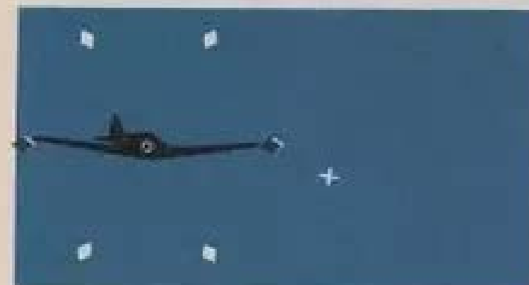
Correct—Circle of diamonds corresponds to target's wing span.
