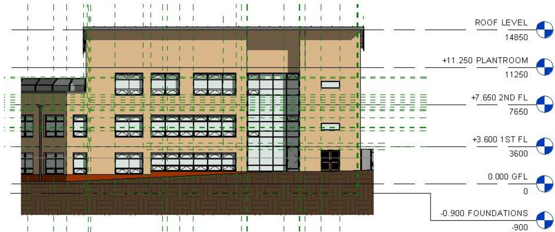
Fig. 25: JSA's Southeast Elevation (Classrooms, Offices, Plantroom)
