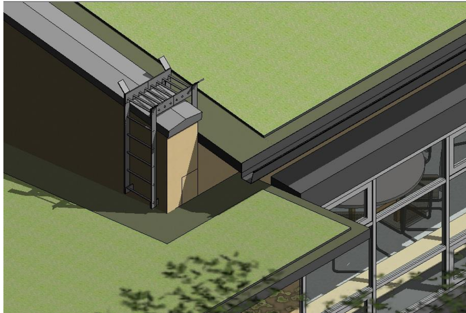
Fig. 17: Roof ladder over the school hall roof
